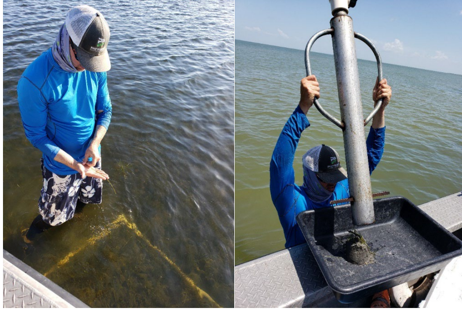
Figure 80. Identifying seagrass species coverage in the 1-m plot (left) and depositing substrate core sample into tray (right).
