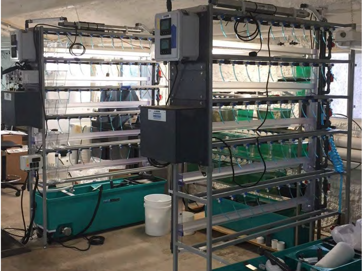
Figure 11. Z-habitat systems used in freshwater mussel propagation during FY-2018 at Ink Dam NFH. Photo Credit: USFWS
