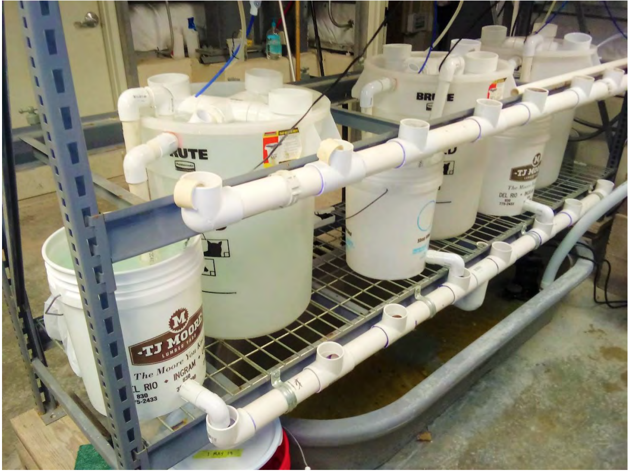
Figure 12. The Up-welling Juvenile Growth System (UJGS) has a pump that recirculates water from a 5-gallon bucket into a 20-gallon basin. To eliminate waste, fresh well water was added from a manifold and excess water exits a standpipe on the 5-gallon bucket that drains down into a basin with a sump pump. The advantage to this system was that three independent systems with three replicates each may be setup to test different feed treatments simultaneously. Photo Credit: USFWS
