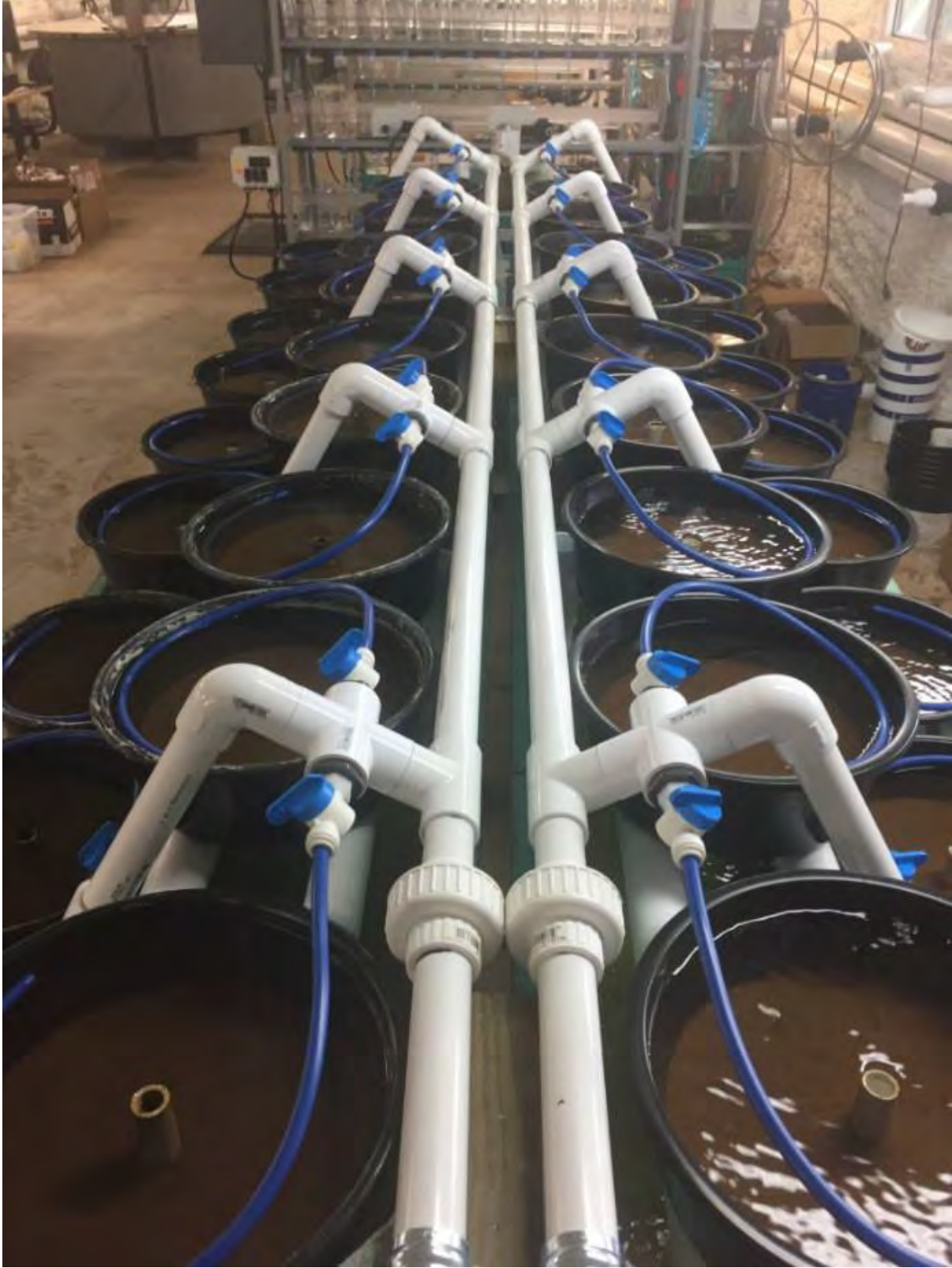
Figure 10. Semi-closed flow-through pan system(s) with total recirculation capability for juvenile freshwater mussel rearing at Inks Dam NFH. Photo Credit: USFWS
