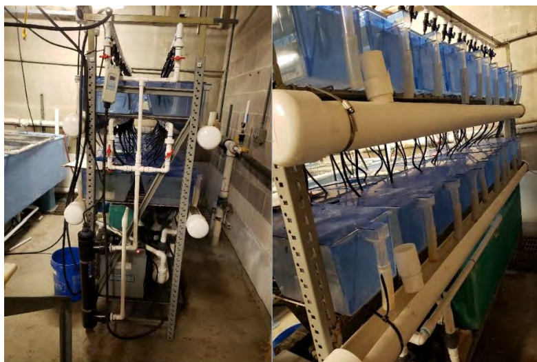
Figure 4. Recirculating (AHAB) flow-through system for holding inoculated fish. Photo Credit: USFWS
