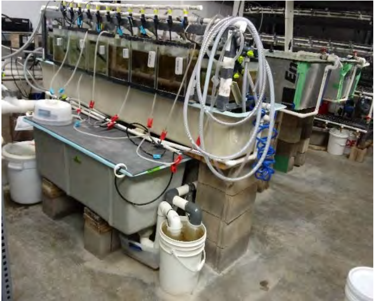
Figure 9. The UNFH mussel culture facility currently has three flow-through systems or Big Blue Habitats (BBHAB1, 2, and 3) designed to maintain large numbers of infected catfish hosts. Nylon collection bags were used to collect high concentrations of juvenile mussels that drop off from large numbers of fish hosts. There are two BBHAB systems below the previously built QAMHAB system. Only one can be seen in this photo. Photo Credit: USFWS
