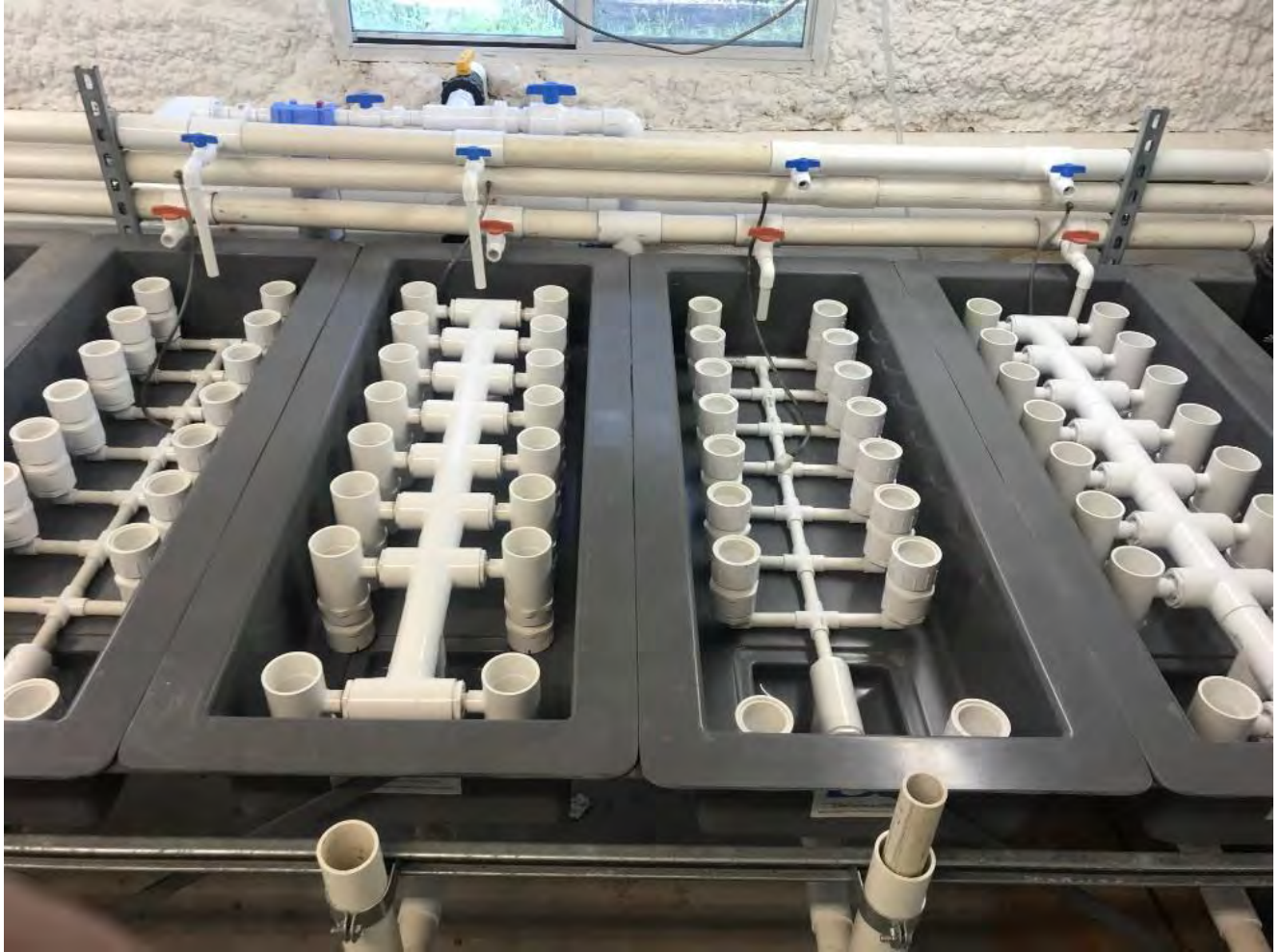
Figure 14. Paired flow-through filtered vs. unfiltered up-wellers and down-wellers. Photo Credit: USFWS
