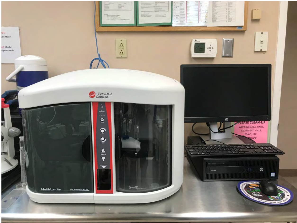
Figure 2: Beckman Coulter Multisizer 4e used to size and quantify particle levels in water.
