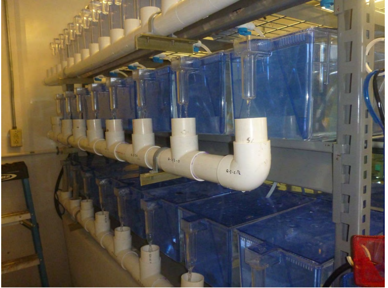
Figure 3: Flow-through AHAB system used to house host fish.
