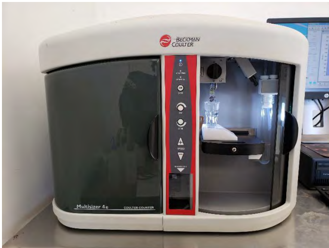
Figure 2. Beckman Coulter Multisizer 4e used to assess the quantity and type of algal cells present in mussel systems and ponds. Photo Credit: USFWS
