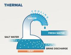
Saltwater is heated up, and the resulting water vapor is condensed and collected.
