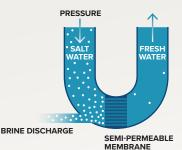
Saltwater is pushed through a series of filtering membranes at high pressure.
