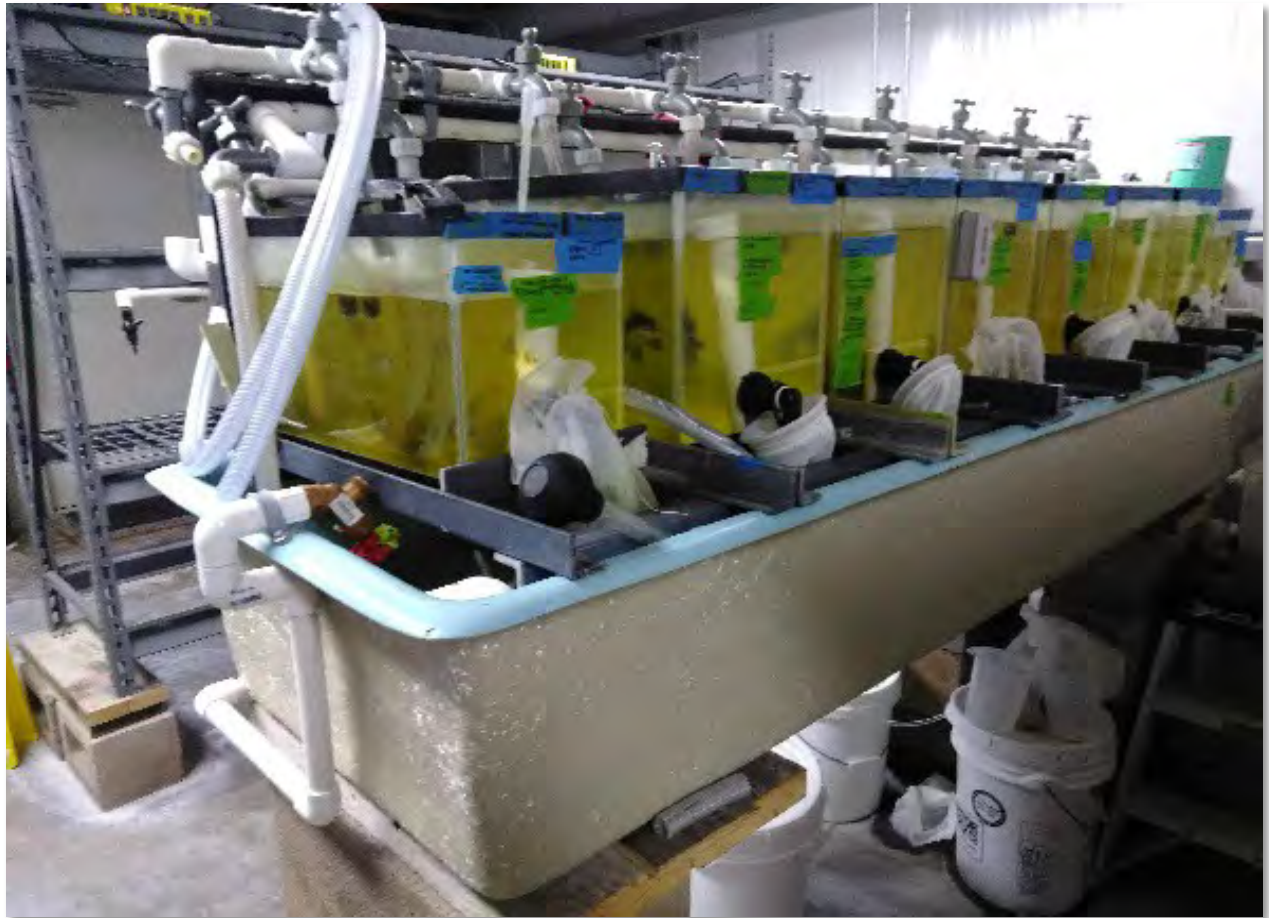
Figure 3. A renovated temperature controlled mussel flow-through system (QAMHAB) capable of holding mussels and fish hosts together for prolonged periods. Photo Credit: USFWS
